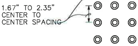
RAISED TRUNCATED DOME DETECTABLE WARNING SURFACE
