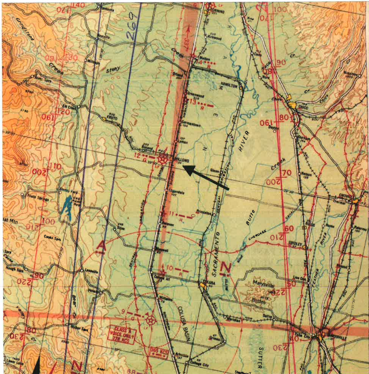
Figure 7 U.S. Army Air Corps Aeronautical Chart, prepared 1930, revised 1933; Air Mail Route identifiers for Willows Airport include “12,” “dot dot dash” (Morse Code for “U”), and “G” (green course lights); chart also shows Beacon 11 to the south near Delevan with an “R” (red course lights) that flashed “W” (dot dash dash) and Beacon 13 to the north, which flashed “V” (dot dot dot dash), also in red
